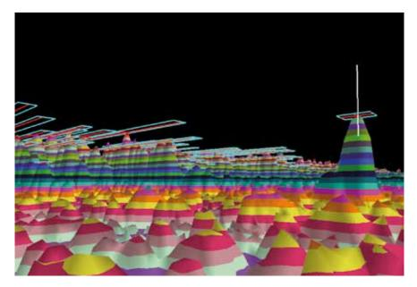
Figure 5 - 3D Doppler view of sea clutter and target
